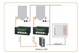
The 5000 can be connected onto a Profibus-DP network with the Rinstrum 1400 Profibus-DP module. The 1400 translates the data from the indicators into the Profibus format. This allows the Profibus master to effectively extract status and weight data for example from the indicators and send commands to the indicators.
